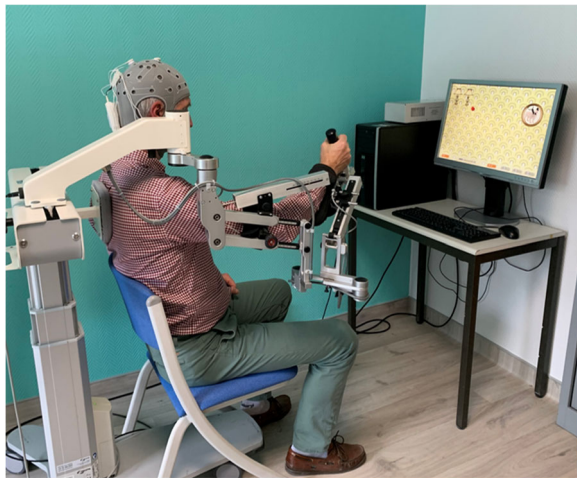
Fig. 2 Patient setup on the ARMEO virtual reality therapy system. The ARMEO exoskeleton counterbalances the weight of the patient's upper limb with springs located on the elbow and wrist joints. The patient is in a resting position, ready to begin to play the ladybug game
